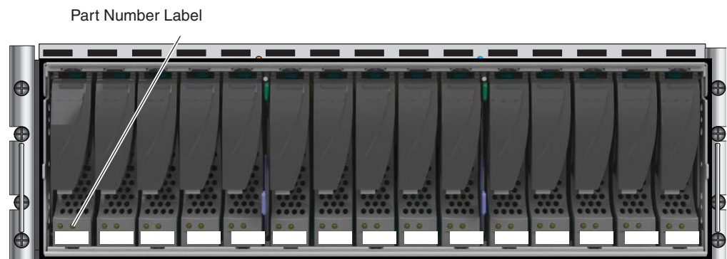
Figure 5 Example of the DPE 3U, 15 (3.5-inch) disk drive (front view)
