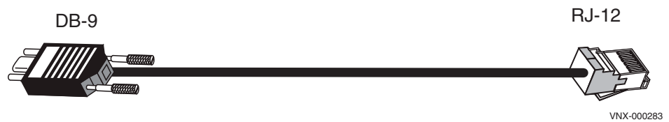
Figure 14 Example of SP A (micro DB-9) to SPS (RJ-12) cable
