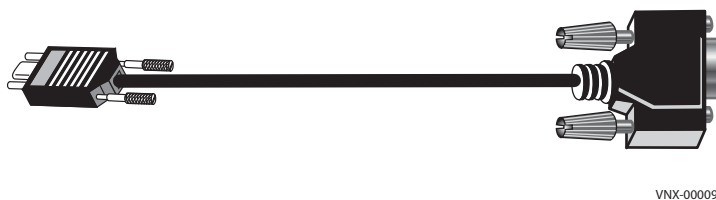
Figure 27 Example of SP null modem (micro DB-9 to serial DB-9) cable
