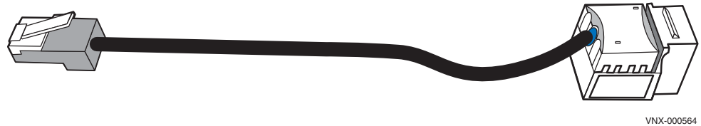
Figure 33 Example of an Ethernet extension (modular plug to modular jack) cable
